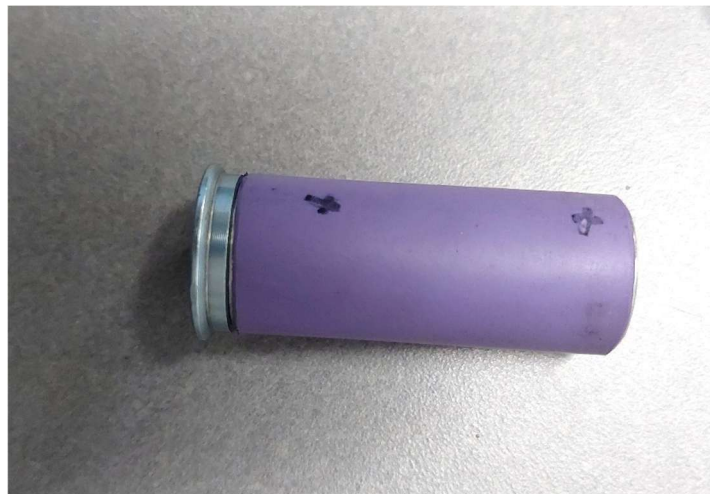
Figure 1: Shell before starting test. X marks the approximate location of dimensional tests.
