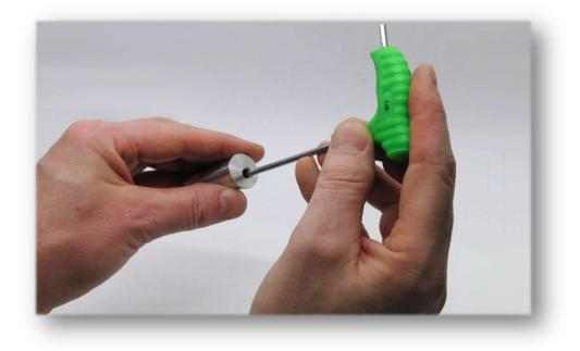
• Should it become necessary to remove the projectile, it can be done by pushing it out using a smaller (~1/8" or about 3mm) Allen Key or similar
