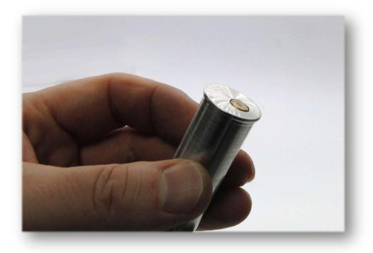
• The rim should generally sit flush and the base can be gently tapped against a flat surface to help or simply loading into a shotgun should achieve the same. Minor protrusion has little effect on the function.
