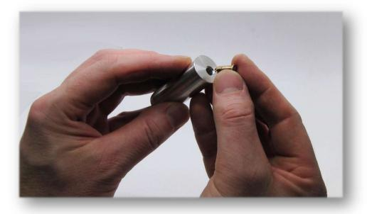
• Loading the .22 Caliber Ramset® Blank is simply accomplished by inserting it into the rear opening. No special tools are required and orientation is not of importance (the rim aligns with the center of the shell)
